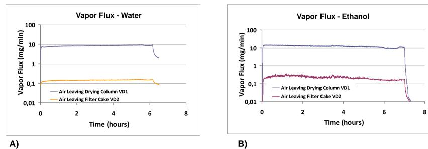
FIGURE 3: Vapor transfer in the drying column during continuous operation. The vapor flux transferred from the drying column to the absorption column is compared with the vapor flux passing through the product filter. A) Water B) 99.5% Ethanol
