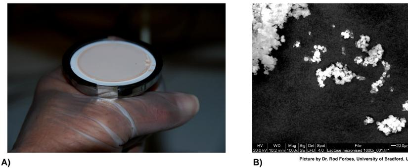
FIGURE 2A: A filter cake of horse radish peroxidase on the 56 mm product filter. B: Scanning electron micrograph of spray dried lactose powder in bulk.
