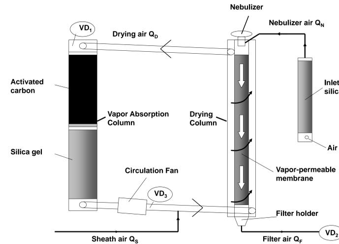
FIGURE 1: A scheme of the LaminarPace spray dryer. VD indicates the positions for the probes measuring vapor concentration/humidity in the system.
