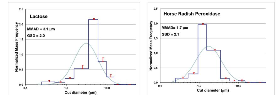
FIGURE 4: The particle size distribution of two spray dried powders aerosolized with the PreciseInhale system.
