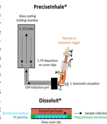
Figure 1. Schematic of the PreciseInhale<sup>®</sup> and DissolvIt<sup>®</sup>
